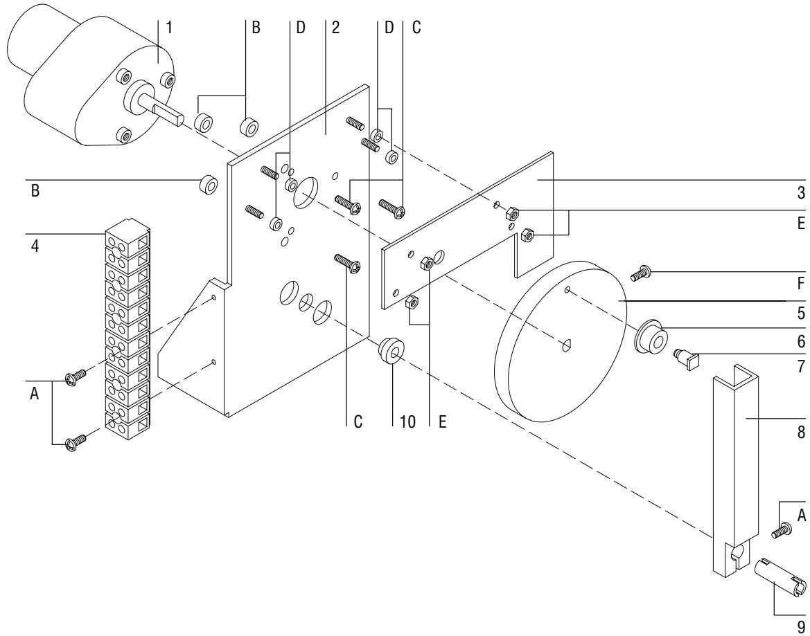
**Figure 5-7.** Six-Port Valve Actuator Assembly
